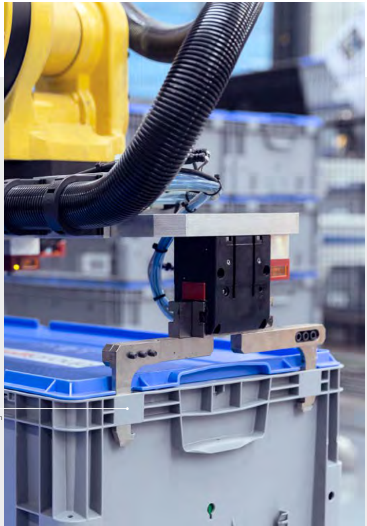
Anthropomorphic robot gripper insertion cavity and weight zero setters.
