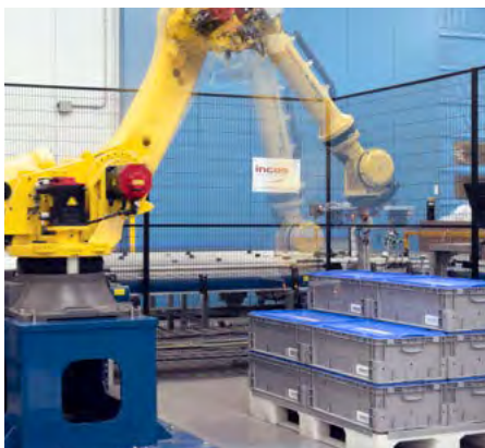
Automatic pallet packing and unpacking station with anthropomorphic robot.
