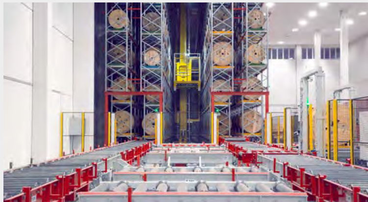
Reel warehouse conveyors.
