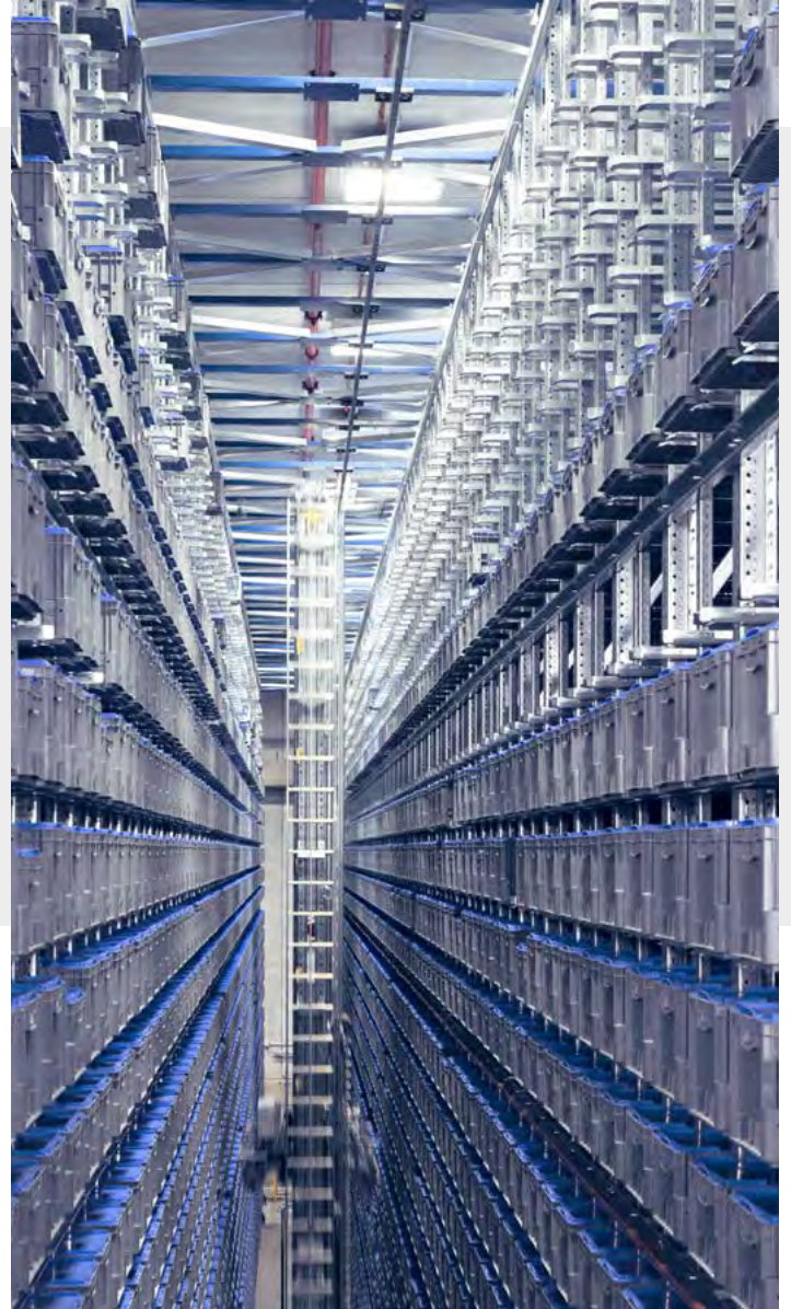
Self-supporting automatic warehouse for boxes with 2 stacker cranes and expansion option.
