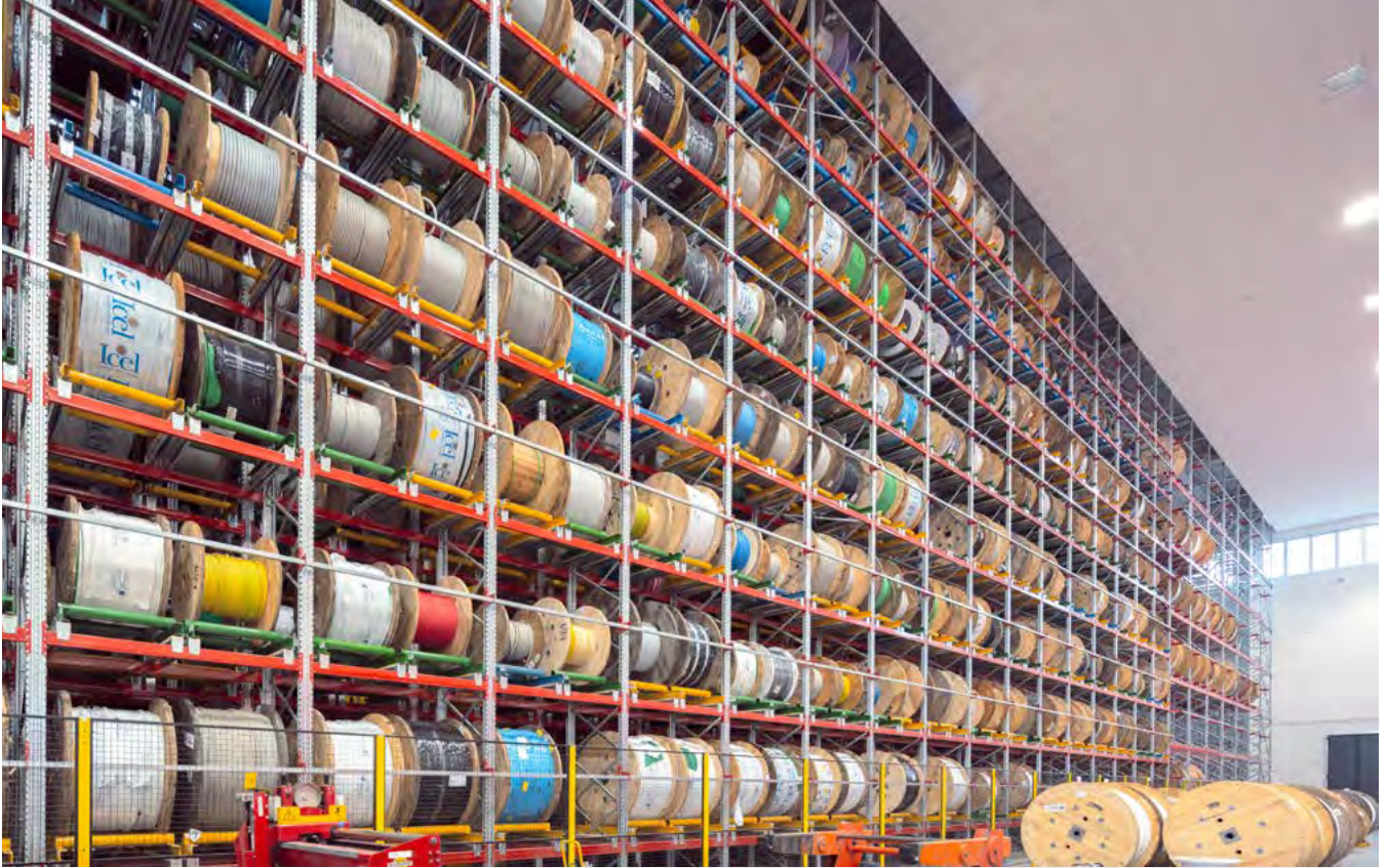
Automatic warehouse for cable reels with dual depth stacker crane.
